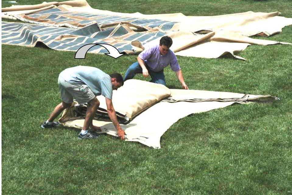
Figure 27 – Fold Fabric Ends onto the Package and Wrap with the Opposite End Fabric
