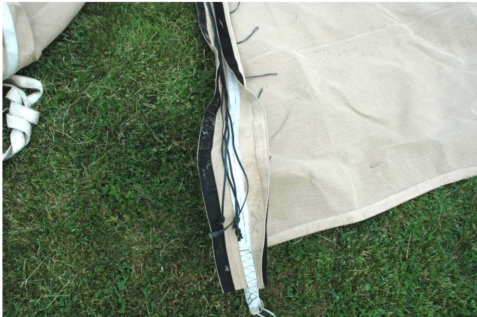
Figure 15 – Secure Output Power Cables in Pocket
